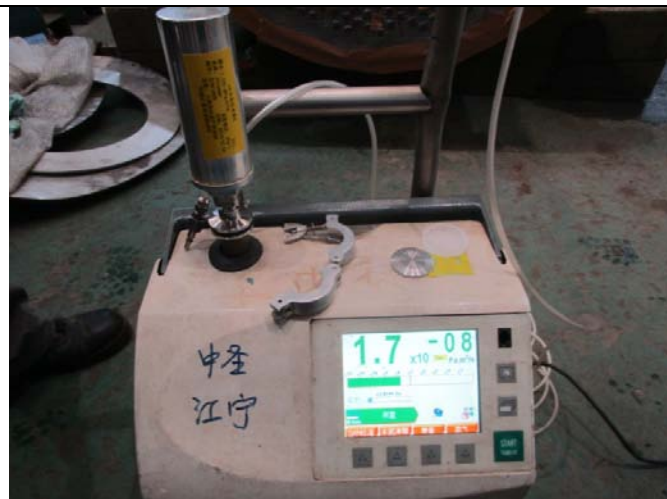
Photo 27. Helium test: Max. helium leak rate
