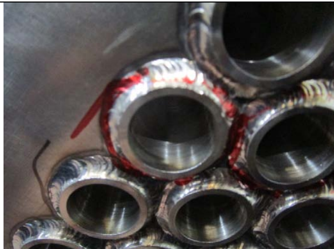
Photo 9. Fitting-up check of nozzle V1&V2
