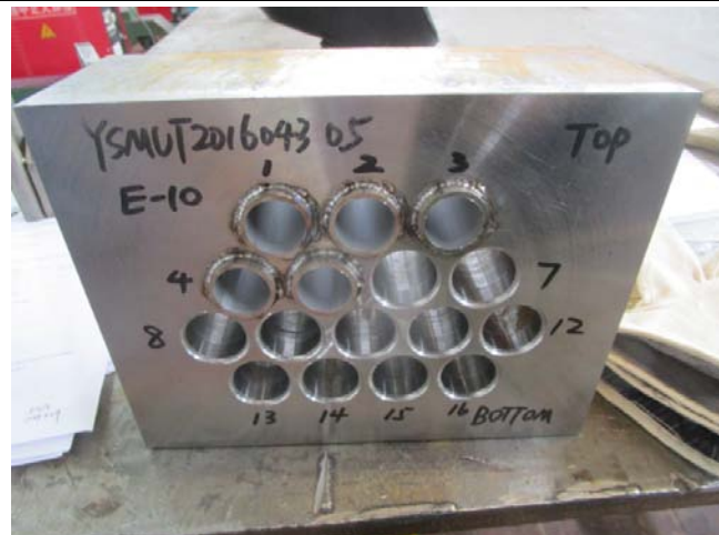
Photo 10. Mock up test: crack was found, YSMUT2016043-5
